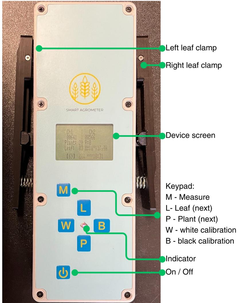
**Figure 1.** Layout of Smart Agrometer keyboard buttons and indicator.
