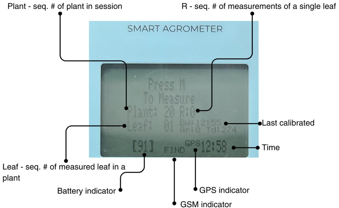
**Figure 9.** Device screen in measurement mode
