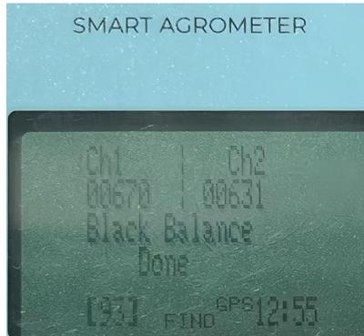
**Figure 3.** Smart Agrometer - Calibration with black
